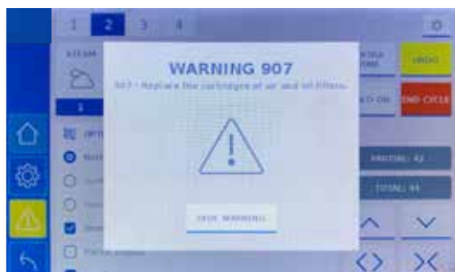
Figure 2.2.5a - Example of due maintenance message.
